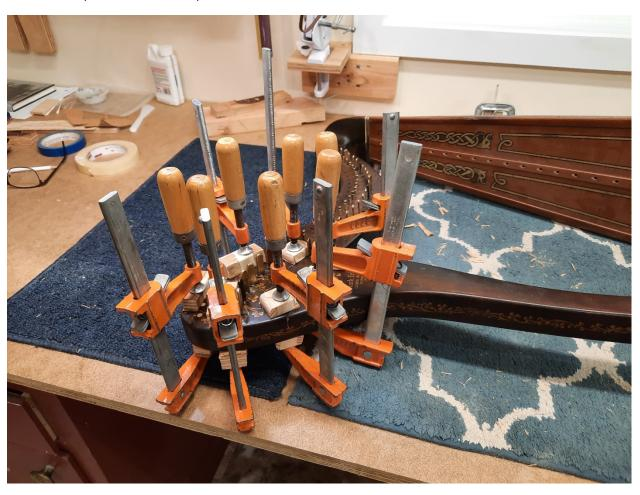
Many of the holes originally drilled to hold the harp's tuning pins were no longer serviceable, so the holes were filled (bushed) and redrilled. Getting the mostly-reassembled harp safely up onto the drill press was an adventure!
